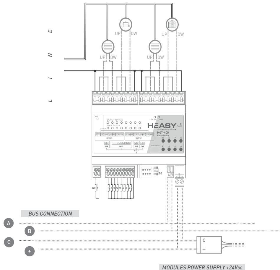
SCHEME 2: Direct wiring for DC motors
