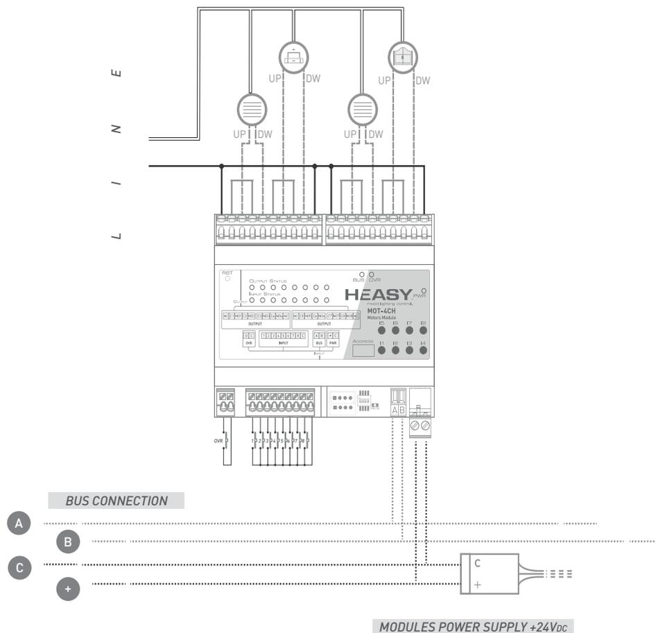
SCHEME 2: Direct wiring for DC motors
