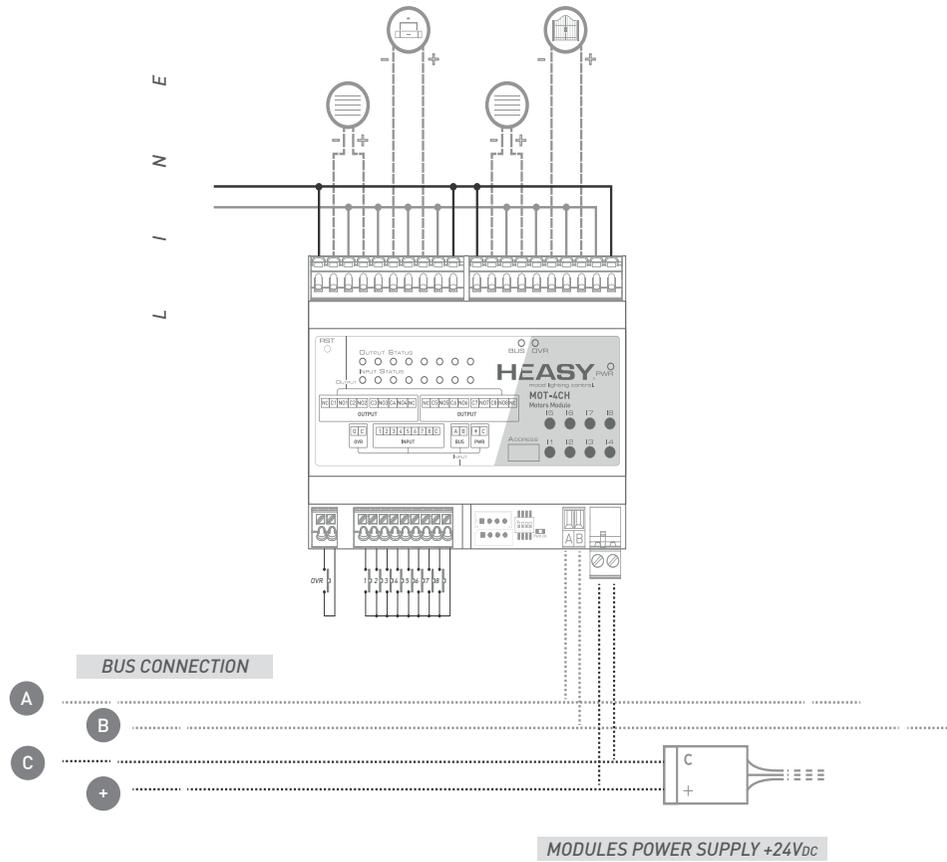
SCHEME 3: Direct wiring for dry contact motors
